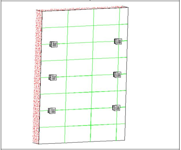
3, use a wrench to tighten 6 body jets on the water outlet holes in a clockwise direction
