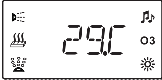
Heating function's model : Long shows is the actual temperature The flicker is the preset temperature
