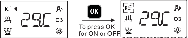
Heating function's model : Long shows is the actual temperature The flicker is the preset temperature
