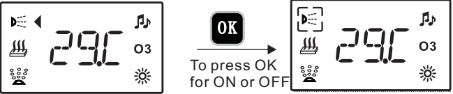
Heating function's model : Long shows is the actual temperature The flicker is the preset temperature
