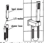
3). Place rubber washers in both ends of the hose. 2). Screw the shower holder clockwise onto the Connect the shower hose to the supply elbow and shower head. Note the ends of shower hose to be connected correctly.
